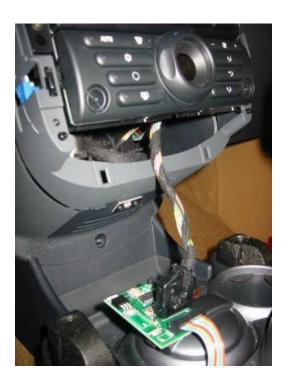
This pic from Bill shows the downtubes removed, the toggle switch panel removed, and the original toggle switch panel connector plugged into the MINI circuit
