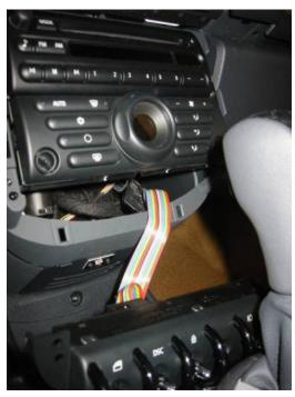
This pic from Bill shows the MINI circuit pushed in behind where the toggle switch panel normally fits, with the harness from it going to the toggle switch panel (the downtubes are still removed)
